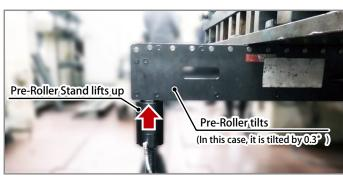
\* The tilt angle will be adjusted during installation.
