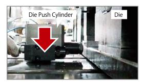
**3** The cylinder is fixed in the T-slot!
