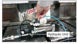
**2** Turn on the switch to supply Hydraulic Pressure!
