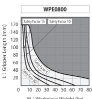
W: Workpiece Weight (kg)
