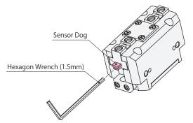
Shapes of sensor dog for opening and closing are different. Please refer to the drawing below and install the sensor dog to the appropriate position. Otherwise, the sensor dog may extremely stick out and/or the proximity switch may not react.
