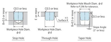
%4. For -T:Taper Hole model, the first gripper ridge is the reference diameter.
