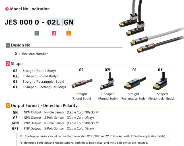
However, for the models WCC, WFC and WHC (marked with %2 in the application table), use two S-pole sensors.
