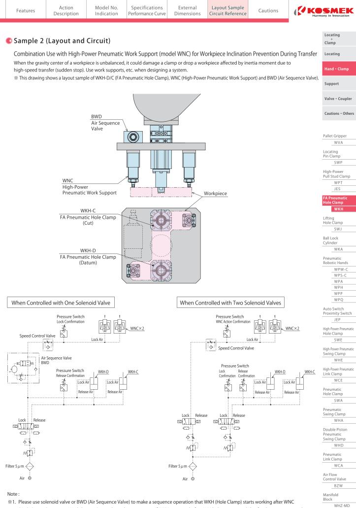
(I. Please use solenoid value or BWD (Air Sequence Value) to make a sequence operation that WKH (Hole Clamp) starts working after WNC (High-Power Pneumatic Work Support) completes the movement. If WKH operates before WNC, there is a possibility for the equipment to be damaged due to a thrust load on WKH.
