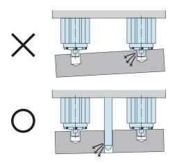
Please set up rough guides considering the pitch accuracy of location clamp / location cylinder mounting hole and each workpiece machining hole when using with another location clamp / location cylinder, etc.
