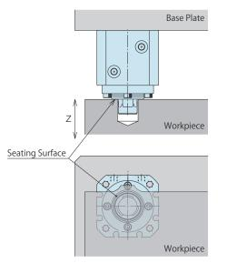
A workpiece must be resting on all seating surfaces when clamping. If not, calculate contacting pressure with clamping force and seating area not to deform a workpiece.
