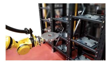
Pallet-Transfer Automation with Articulated Robot
