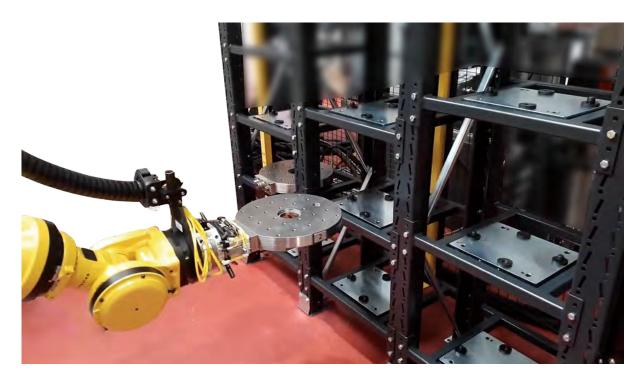
Pallet-Transfer Automation Example using Articulated Robot
