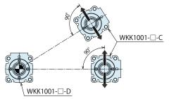
⇒ shows the expanding direction of the gripper.
