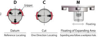
lpha When roughly locating a workpiece with workpiece hole code 060  $\sim$  085, refer to "Hole Gripper Installation" on P.25.
