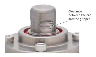
Minimal clearance between the cap and the gripper prevents cutting chips from entering inside the hole gripper.
