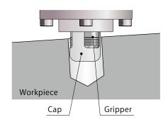
The cap prevents the gripper from frictional wear when inserted to a workpiece hole.
