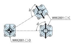
shows the expanding direction of the gripper.
