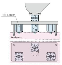
■ Workpiece holding stroke is short to allow for quicker gripping cycles. Eliminating interference enables robots to operate in a smaller footprint, leading to overall reduction in transfer time.
