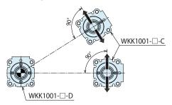
→ shows the expanding direction of the gripper.
