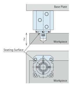
A workpiece must be resting on all seating surfaces when clamping. If not, calculate contacting pressure with clamping force and seating area not to deform a workpiece.
