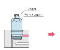
Release Hyd. Pressure : ON Lock Hyd. Pressure : OFF
