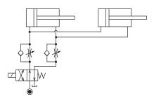
[Meter-in Circuit] (LKE/TLA/TMA/TND must be controlled with meter-in.)
