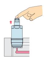
Release Hyd. Pressure: OFF Lock Hyd. Pressure: ON
