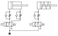
○ Reduce the influence of double acting cylinder control unit. However, due to the back pressure in tank line, single action cylinder is activated after double action cylinder works.
