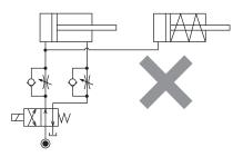
Refer to the following circuit when both the single acting cylinder and double acting cylinder are used together.
