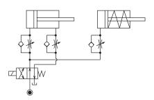
② In the case of meter-out circuit, the inner circuit pressure may increase during the cylinder action because of the fluid supply. The increase of the inner circuit pressure can be prevented by reducing the supplied fluid beforehand via the flow control valve. Especially when using sequence valve or pressure switches for clamping detection. If the back pressure is more than the set pressure then the system will not work as it is designed to.
