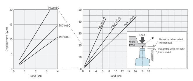
※ The Displacement of TND-Q: Long Stroke Model is larger than that of TND: Standard Model.
