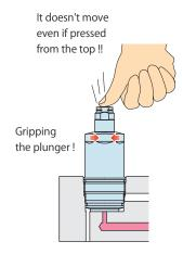
Release Hyd. Pressure: OFF Lock Hyd. Pressure: ON
