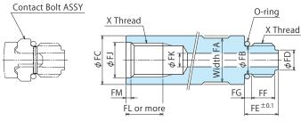
\*\* When a longer contact bolt is required, design it according to the contact bolt adapter design dimensions.
