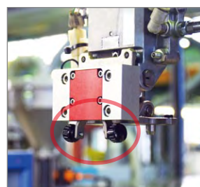
Ex. 1) Making arms thicker so that it is easier to push.
