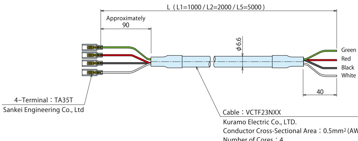
※A crimp tool for crimping the applicable terminal (TA35T) is required when preparing a cable by yourself referring to this drawing.
