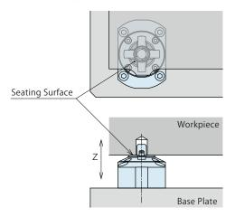
When clamping, make sure all seating surfaces touch a workpiece. When the workpiece is not touching the seating surface area, please refer to external dimension chart and calculate contacting pressure with clamping force and seating area not to deform the workpiece.
