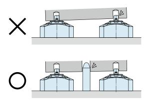
When using the product with other locating clamps or locating devices, please set rough guides considering the center distance accuracy of each mounting hole and workpiece hole of locating clamps or locating devices.
