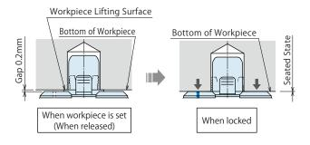
With lifting function, when workpiece is set (before supplying lock hydraulic pressure), the workpiece is lifted up by built-in spring, and there will be a gap of 0.2mm between workpiece bottom surface and seating surface.
