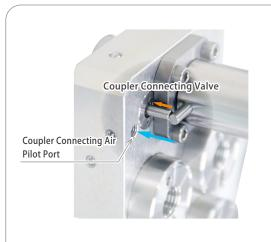
Pilot air is always connected since the coupler connecting valve is opened as JMC: with Check Valve is connected. Check valve for coupler connecting valve is not required.
