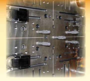
The ejector rod has been divided into a base rod and an attachment rod for speed, simplicity and ease-of-use when changing ejector patterns. No tools are required, allowing changes in mere seconds.
