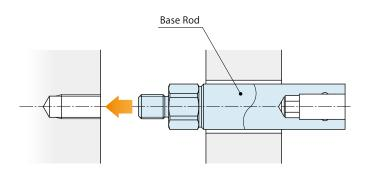
The base rod can be tightened using a hex key.
