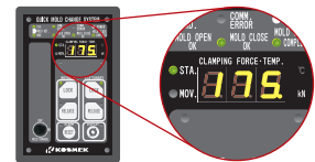
Clamping force displayed on the control panel.
