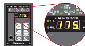
Clamping force displayed on the control panel.
