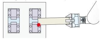
It is unable to secure the clearance for loading the irregular-shape workpiece.
