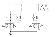
O Reduce the influence of double acting cylinder control unit. However, due to the back pressure in tank line, single action cylinder is activated after double action cylinder works.
