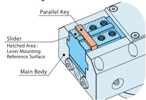
When the parallel key is installed.
