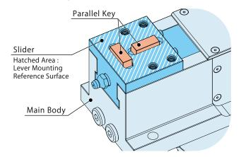
When the parallel keys are installed.
