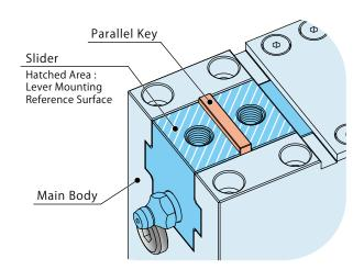
When the parallel key is installed.
