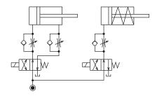
○ Reduce the influence of double acting cylinder control unit. However, due to the back pressure in tank line, single action cylinder is activated after double action cylinder works.
