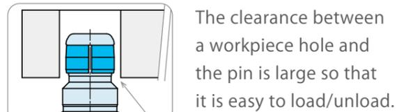
The clearance between a workpiece hole and the pin is large so that it is easy to load/unload.
