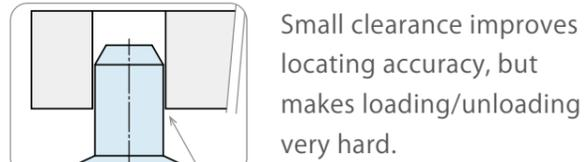
Small clearance improves locating accuracy, but makes loading/unloading very hard.
