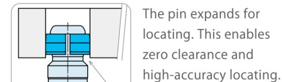
The pin expands for locating. This enables zero clearance and high-accuracy locating.
